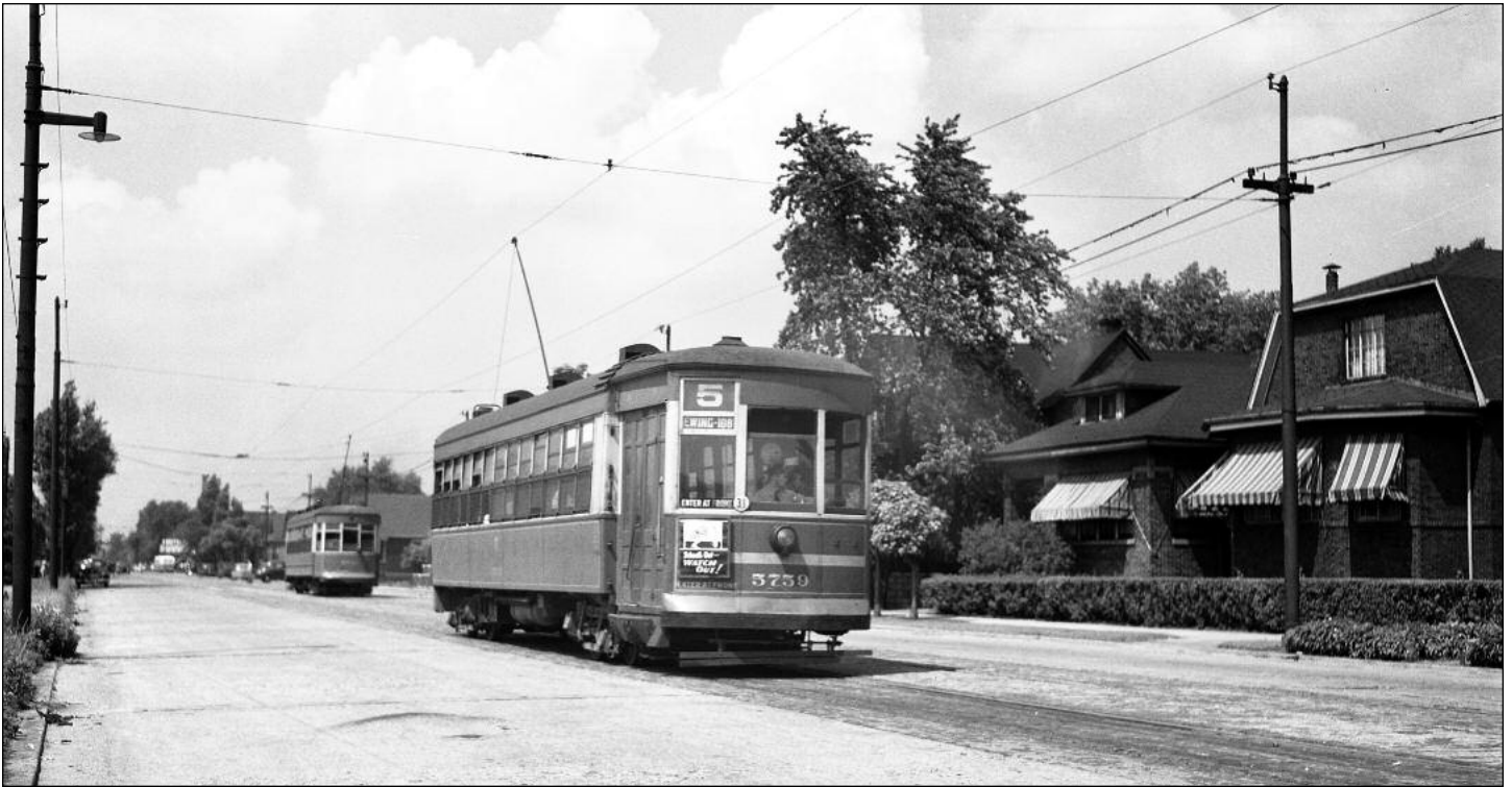
▲ On July 13, 1947, CSL Nearside 5759 is southbound on Ewing Avenue near 108th Street on the last day of Route 5 Cottage Grove-South Chicago service south of 93rd Street. The Chicago City Railway streetcar was built by Brill in 1912 and is running on Calumet & South Chicago tracks.— Robert W. Gibson photo, W.R. Keevil Archive
