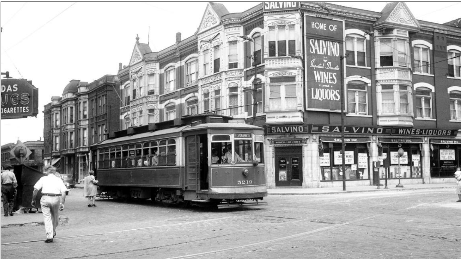
▼ Southbound on Halsted Street at Taylor Street on trackage of Chicago Railways, CSL Big Brill 5219 was built in 1906 in a 400-car order for Chicago City Railway. This photo on Route 8 Halsted in spring 1947 illustrates the integrated operations: a streetcar of the South Side company running on rails of the North Side company on the West Side of Chicago.— Fielding Kunecke photo, W.R. Keevil Archive
